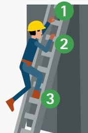
Maintain three points of contact at the working position. Always grip the ladder and face the ladder rungs while climbing or descending.
