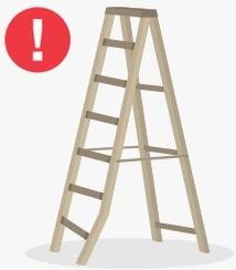
Before using a ladder, inspect it for defects such as, broken rungs or rails. Ladders shall have non-conductive siderails if they are used where the employee or the ladder could contact exposed energized electrical equipment.
