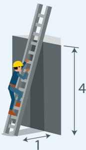
Ladder angle should be at the safest position to work from - Erected at correct angle (4 up to 1 out).
