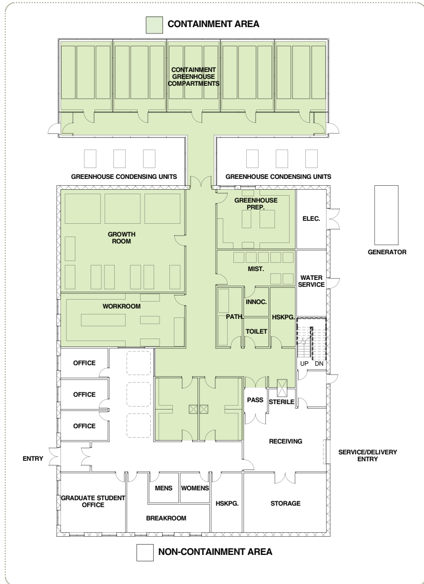
FIGURE 7. Typical Containment Facility Floor Plan*
