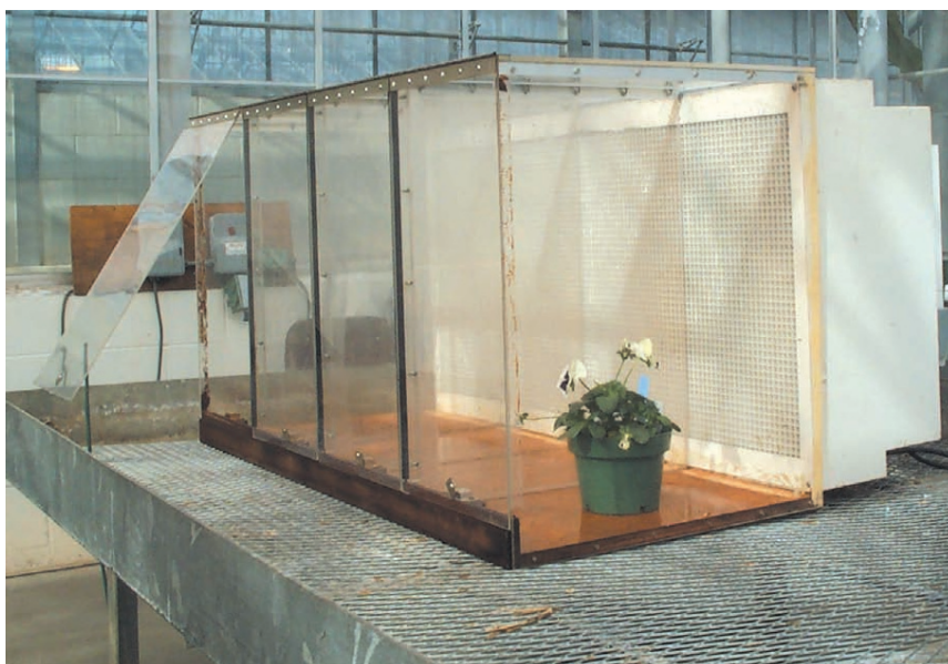
FIGURE 2. Negative Pressure Bench-top Containment Unit
