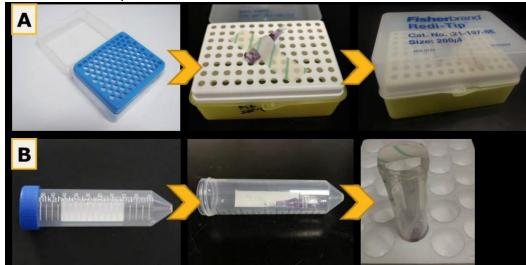
Option A: Obtain a pipet box -> Place biological indicator and keep in place with autoclave tape -> Close the lid
