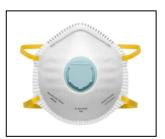
FFRs are divided into classes based on their filtration capabilities. "N95" is a term referring to the N95 filter class, which removes at least 95% of airborne particles using a "most-penetrating" sized particle during "worst case" testing. The FFR classes include N (not resistant to oil), R (somewhat resistant to oil), and P (strongly resistant to oil) series, which are available at 95, 99, and 100 filtration efficiency levels.
