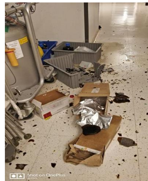
Explosion of hazardous waste bottle causing chemical contaminated debris and spill in the service corridor.
