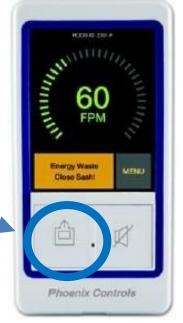
\* Press button to increase the ventilation of the fumehood. Press again to return to normal.
