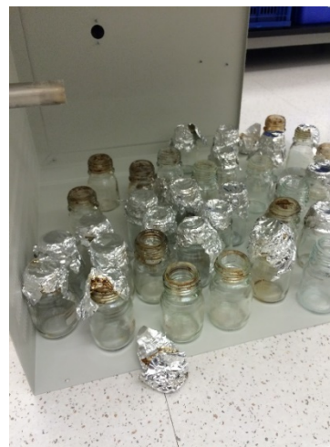
Bottles depicting plastic pour ring residue after burnout
