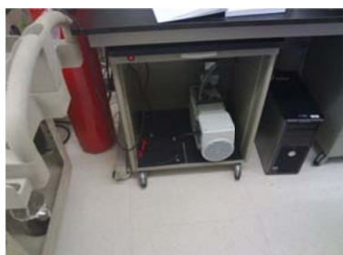
Figure 14: The vacuum pump is too large for the C3 cabinet. The vents at the back of the cabinet are blocked by the utility carrier.
