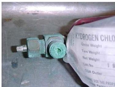
Corroded valve on a hydrogen chloride lecture bottle.
