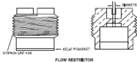
Figure 1: Restrictive Flow Orifice
