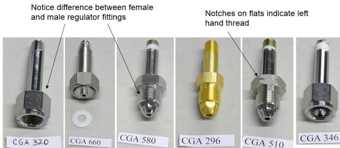
Note the difference between the male and female regulators. Also note the different types of material for different types of gas. Notched flats mean a left hand thread. Used for flammable and some oxidizing gases.
