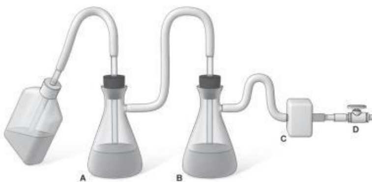
The left suction flask (A) is used to collect the contaminated fluids into a suitable decontamination solution; the right flask (B) serves as a fluid overflow collection vessel. An in-line HEPA filter (C) is used to protect the vacuum system (D) from aerosolized microorganisms.
