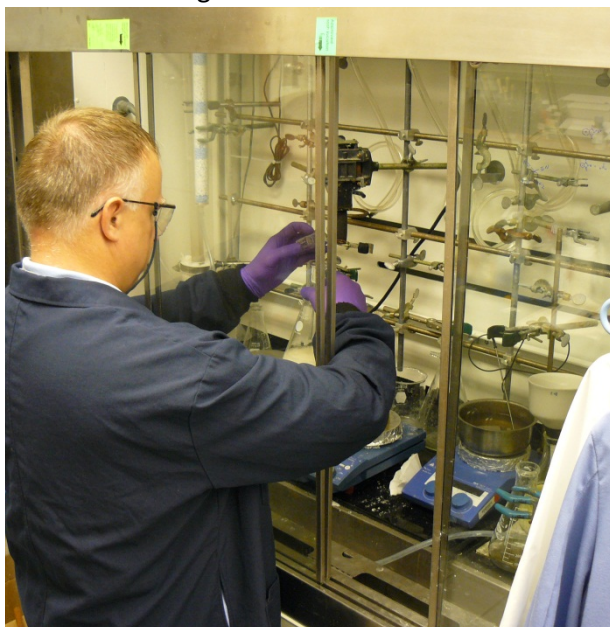
Researcher using hood sashes as a shield
