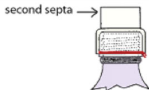
Fig. 1B For long-term storage, use a second septum
